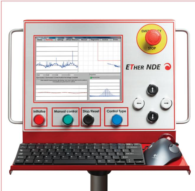
**EXCELLENCE IN CONTROL:** The VEESCAN Control Panel is a stand-alone unit to ensure the safety of the inspection team and offer ease-of-use with the ability to position it freely.
