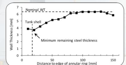
The above graph represents an example result of an annular ring inspection with the MAXWELL PECT, showing severe wall loss close to the tank shell. The corroded area extends over a length of about 80mm (3.15ins) in this case.
