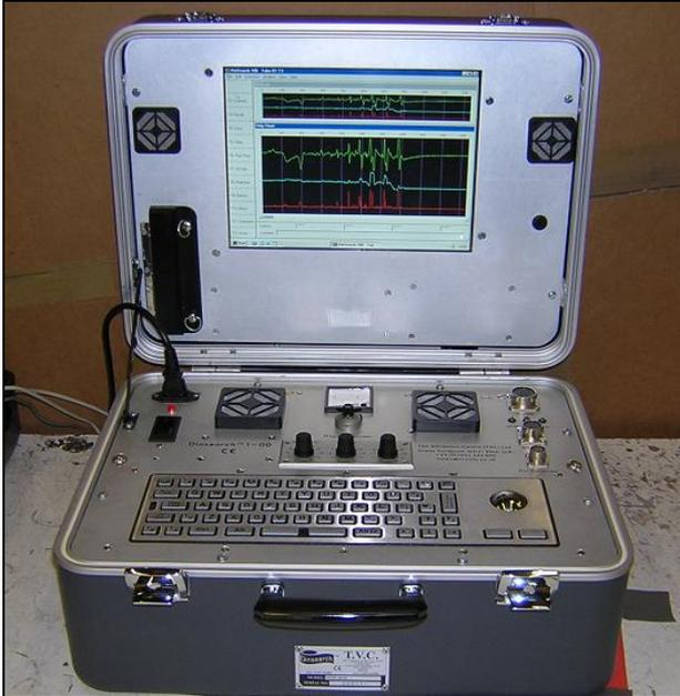
DINSEARCH 1-00 is an electromagnetic system for rapid, high resolution inspection of carbon steel tubes in heat exchangers, coolers, boilers and similar equipment.
